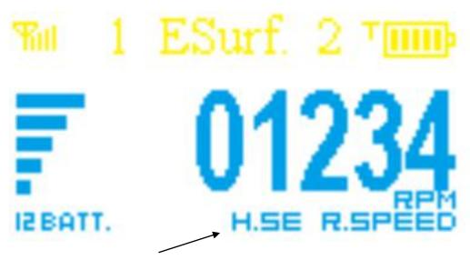
Motor RPM is detected by one hall sensor wire.
