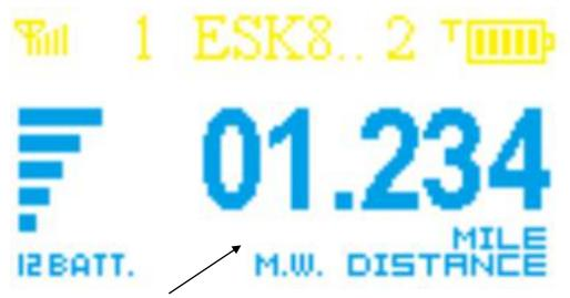
Distance is calculated based on RPM detected by one motor phase wire and showed in Mile.
