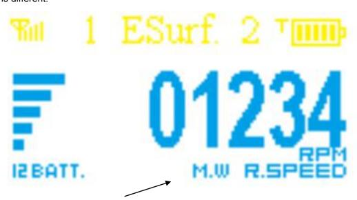
Motor RPM is detected by one Motor phase wire.
