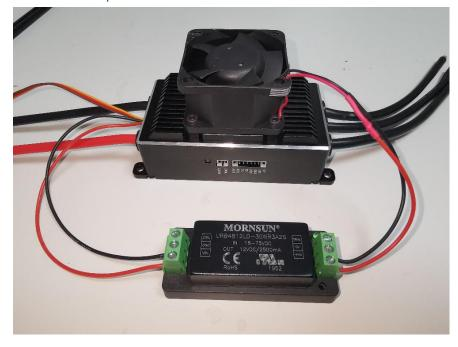
3.6 After checking all in good and correct connection, connect the ESC to a power supply above 18V. After one second of power-on, the fan starts to run. Be careful not to touch the fan blades.
